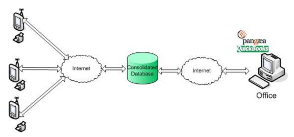
Each user has a SVS handheld computer and (optional) wireless printer. The information relevant for everyday operations is stored in the handheld's database.
